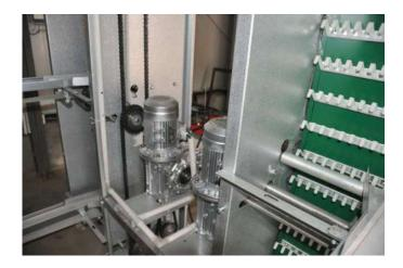
Egg collection system made by the vertical egg collection machines and egg conveyors.
