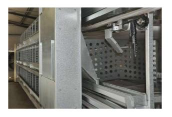
Both of the traveling hopper machines or the chain feeding system are available.
