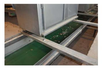
A cover has been placed at back of the manure belts for avoid splashing and not to make dirty hen house and transfer the manure to the conveyor as dandy.
