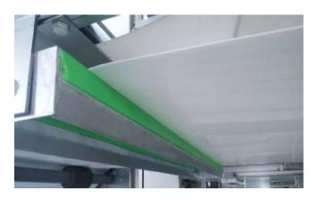
Manure is cleaned and discharged by the Polypropylene (PP) manure belts of 1.10 mm thickness.
