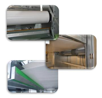
After first cleaning, we have added the second scraper device, it's making the manure belt very clean. The second manure scraper designed in adjustable way according to chicken manure thick
