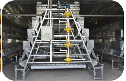
Easy for pullets to get water from special designed nipple drinker, nipple drinker with cup can prevent water from dripping on the pullets and endanger the health of pullets.
