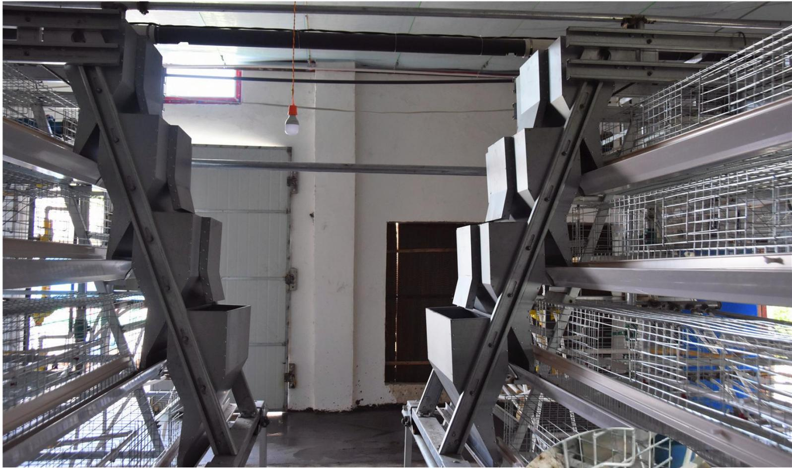
Feeding hopper is connected by rivets without welding, making it more durable.
