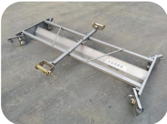
The manure dropping from the cages in the manure pits, and the scraper can collect the manure from manure pits to the outside of house.
