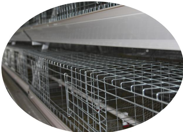
Both the cage meshes and cage stands are made by hot galvanization steel, which ensure the chicken cage can withstand the corrosion of chicken manure for a long time, the service time of the chicken cage can reach more than 15 years.
