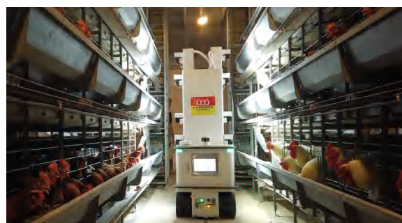
Chicken house inspection robot (SHEEPDOG)
