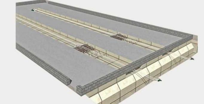
The machines in each row can operate independently, making it easier to remove chicken manure in any row
